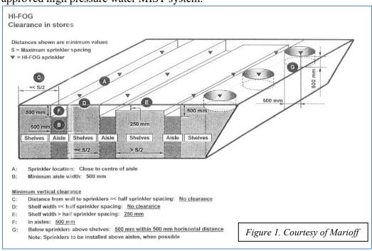
a. If MIST nozzles are placed in EACH aisleway created by shelving and the nozzles are spaced within the maximum allow spacing distance (S), determined by the system
